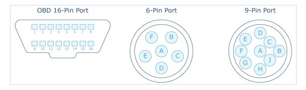
**\* NOTE:** A standard GO9 device is also a 16-Pin Port, so a harness may not be required.
