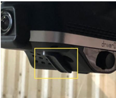
3. Initiate a Power Cycle by pulling the power plug on top of camera.
