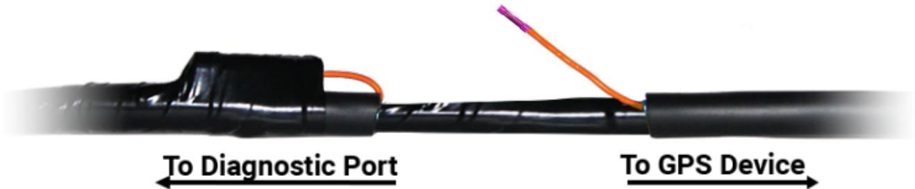
Remove 1 in. of sheathing from the inline fuse holder and butt connect the fuse holder to wire leading to the GPS device connection before taping off and cable tying connection.
