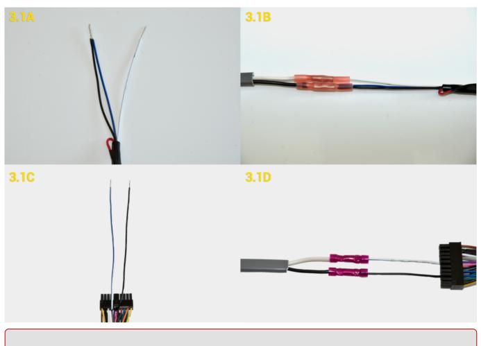
**Note.** Heat must be applied to every heat-shrink butt connector to ensure there's a water-tight seal. When applying heat, glue will seep from the butt connector; do not overheat the connection as this can cause damage to the wire or surrounding wires.
