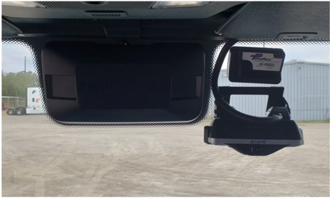
Mounting examples towards the passenger side (here right) of the CAV/LDW Device
