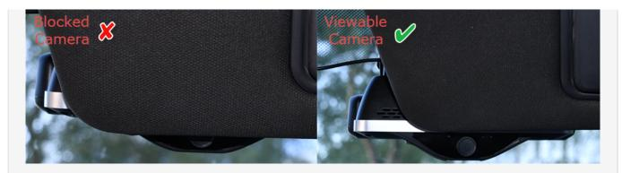
• Type 2: Rear View Mirror (Sensor Housing/Large Trim); Right side of housing/trim with bracket bottom the same level as housing.
