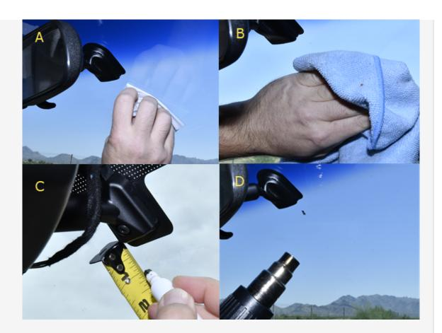
**Note.** Excessive heat may cause delamination of the windshield or cracking. Continuously move heat gun to not apply heat in one area for too long.
