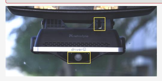
1. Place the device into the mounting bracket and lightly screw in the mounting bolts. Do not fully tighten down screws as the camera may need to be adjusted in Step 3.
