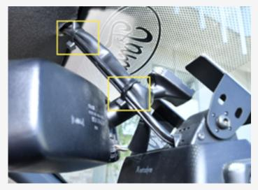
4. Route the antenna cable between the windshield and a-pillar plastic. Remove the VHB plastic exposing the adhesive, and press the antenna to the dashboard. Once complete, put the a-pillar plastic back into place.
