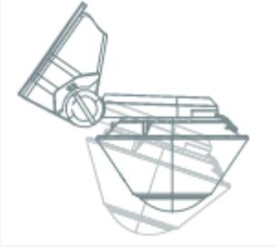
3. Tighten the Dock into place by turning the adjustment slot clockwise with a coin.
