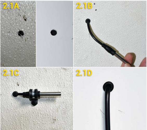
2. Using cable ties, secure the temperature sensor cable every 1 1/2 ft. as you route the cable from outside to inside the cab, and behind the dashboard cluster.
