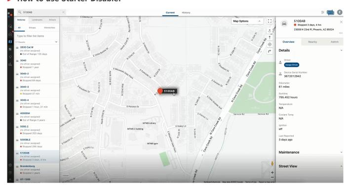
1. From the Portal, use the Vehicle List (left-hand panel) or the Search field to locate the vehicle for which you would like to disable the vehicle's starter.
